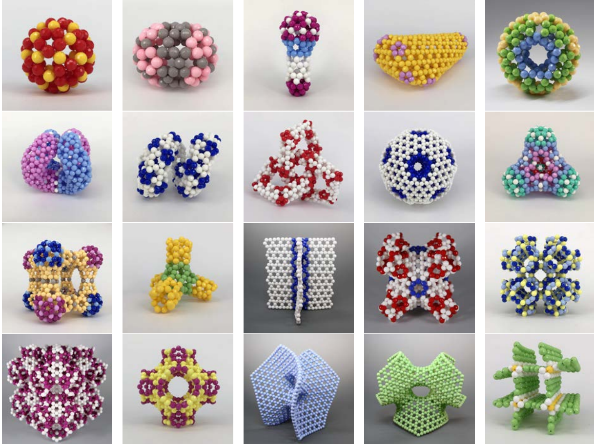
Figure 3: Curved graphitic structures. First row: Buckyball ( C_{60} ), endcapped carbon nanotube C_{80} , fullerene with lollipop shape, HIV virus, carbon nanotorus C_{120} ; Second row: curved nanotori, helically coiled carbon nanotube, carbon trefoil knot, dodecahedral high-genus fullerene, genus-3 carbon tetrahedron; third row: fused C_{60} cube, carbon tetrapod, single periodic minimal surface, I-WP surface, (1, 0) -P-surface; Fourth row: (1, 1) -P-surface, (2, 1) -P-surface, Chen-Gackstatter surface, a genus-2 surface, intersection for four graphene sheets with four lines of sp^3 defects.
